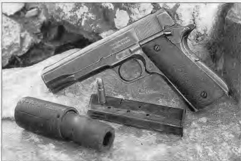
Probable Viet Cong jungle workshop conversion of M1911A1 pistol to caliber 7.62x25mm. Shown with VC hand grenade.
